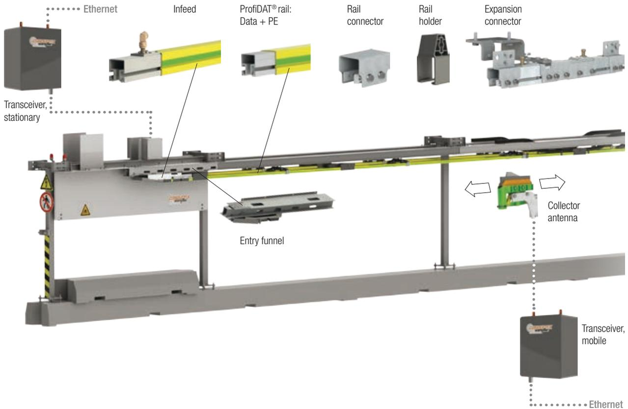
The ProfiDAT® data transmission system for E-RTG cranes is a variable length system used to provide communication between the stationary feed point and the mobile drive-in unit of RTG container cranes. The ProfiDAT® system is installed in parallel with the E-RTG/RTG electrification system, which is a current collector system for container-stacking cranes.
