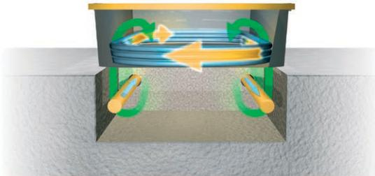
The secondary Pickup is able to move freely. It can be positioned with an air gap and sufficient tolerances in relation to the primary conductors and can also move at any speed.
