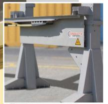
The short Drive-In zone allows the E-RTG to run with electrical power from the very first container row.
