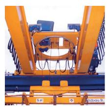
Supply of the turning-crab on an EOT-crane
