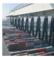
Supply of the crab on a fast travelling STS-container crane
